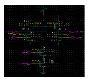
Figure 3. Modified MCML Inverter
