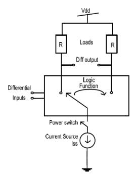
Figure 1. Basic MCML logic circuit
